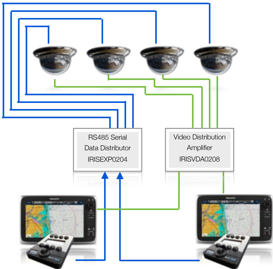
Fig:2.0. Slightly more complex set up with 4 IRIS106 cameras being controlled and viewed at 2 separate helm positions. Data from each controller is fed into the input of the RS485 Serial Data Expander, and data to each camera is connected to the outputs. This keeps the data 'clean' and prevents data cross talk and over-runs. Video from each camera is fed into a VDA (Video Distribution Amplifier), which feeds two MFD's. Power not shown to keep diagram simple.
