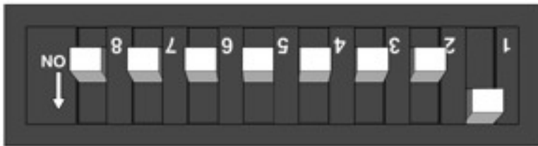
Fig.3.0: Example of Camera Address set to 1
