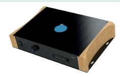
Central to any on board CCTV and security system is the digital recorder. Iris's new range of hybrid recorders are designed with solid state technology to make them suitable for use on board boats of all sizes and other mobile applications. Each model is housed in a moisture proof enclosure and waterproof field connectors are supplied.
