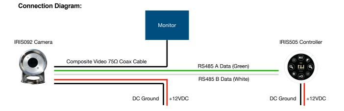
Power Note: The IRIS092 draws less than 200mA. Please ensure the DC power to the camera is protected by a suitable fuse or breaker.
