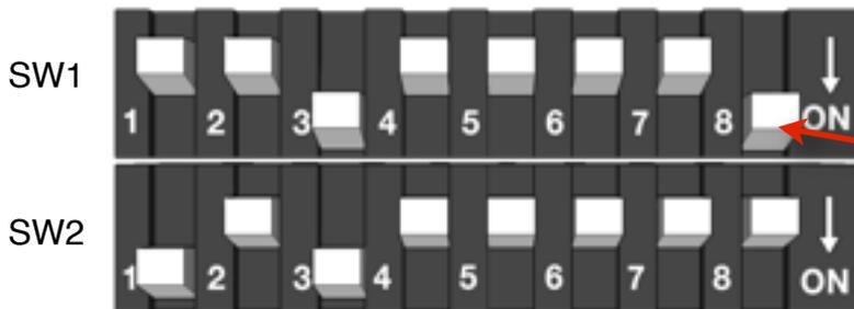
When Bank 1 Switch 8 is set from OFF to ON the video output will flip to the 'ball down' orientation and the cameras memory will be activated. This stores any subsequent image flip command sent from the IRIS595 controller.
