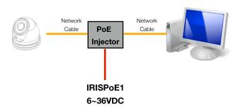
Use a standard 568B ethernet CAT5 cable to hook your computer up to the PoE injector, and then another 568B cable to hook the camera up to the injector.
