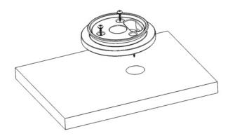
Present your cables to the camera through the cable entry hole you've just drilled. If you have a PoE version of the camera, this will just be a single CAT5 cable. If you have a non PoE version, you will need a CAT5 cable and 2 cores 18AWG for the DC power. Ensure terminations are sufficiently protected from any moisture ingress. Details on how to fit the waterproof plug are on the next page.
