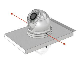
FULLY LOOSEN PRIOR TO ADJUSTING INNER DOME POSITION (BOTH SIDES OF CAMERA)
