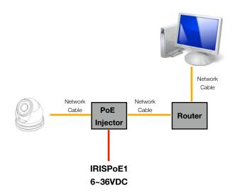
As mentioned previously, the camera as default is set to obtain its IP address automatically via DHCP. This means that once connected, your router will detect the device and assign it an IP address within its designated range (refer to the documentation for your router for further details). You must also ensure the network adapter for your computer is set to obtain its address via DHCP.
