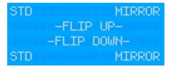
FLIP UP refers to the standard 'desktop' orientation. The MIRROR option will flip the image horizontally (useful when using the camera to look backwards). FLIP DOWN refers to the camera in the hanging orientation.
