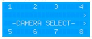
Select the desired camera (1~8) or move the joystick RIGHT to access cameras 9~16. Once the desired camera is selected the controller will return to the HOME screen.
