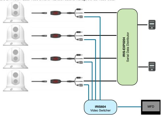
Systems can be expanded by using Serial Data Expanders to manage the control data and Video Distribution Amplifiers, Video Switchers or Matrices to manage multiple video feeds. In addition, IP encoders can be added to enable connection over a computer network so cameras can be viewed and controlled from smart-phones, tablets and computers. For further information or to discuss your requirements, please contact Iris.
