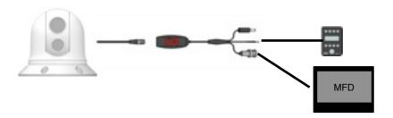
If there are multiple cameras, controllers or other PTZ cameras on the system, it will become necessary to add a serial data distributor in order to balance the data and ensure there are no signal reflections that could result in over-runs and poor camera control. Below is an example of a system with 2 controllers and 4 cameras. An IRISEXP0204 data expander has been used to manage the data cables, and an IRIS604 Quad Video Switcher has been used to manage the four video feeds.
