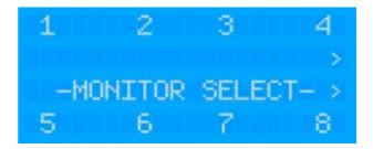
Select the desired monitor (1~8) or move the joystick RIGHT to access monitors 9~16. Once the desired moniitor is selected the controller will return to the HOME screen.
