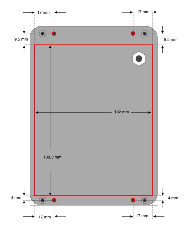
The IRIS516 is designed to be panel mounted into a suitable dashboard or helm.
