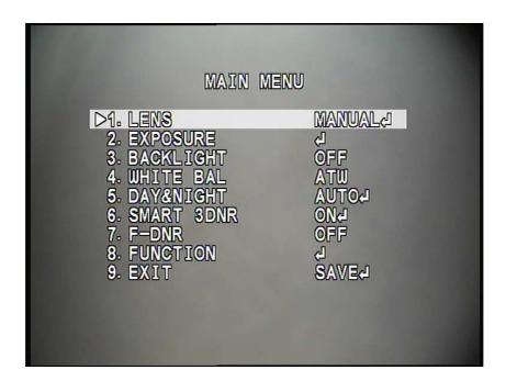
The menu can be navigated using the joystick up, down, left and right, and by clicking the joystick in its centre position to select an item. Any item with an arrow at the end of the text indicates that there is a sub-menu available by clicking the joystick, and anything without the arrow can have it's options changed by simply moving the joystick left or right. The Return option at the bottom of each menu returns to the previous menu.
