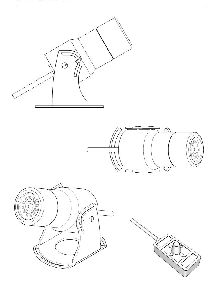
The IRIS090-IR is designed to be ceiling, floor or wall / bulk-head mounted and is affixed using the supplied mounting screws to the required surface.
