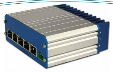
The new IRIS-PoE4 is a compact four channel power over ethernet (PoE) injector designed and certified especially for use in vehicles, marine and solar power applications.
