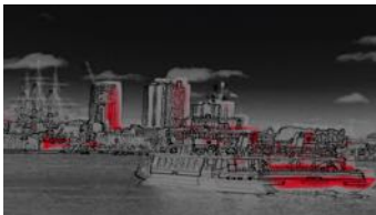
Fusion Mode A - ICE+ Edge Enhancement From Daylight Camera overlaid onto thermal image)
